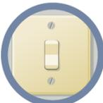
Switches are used to break an electrical circuit. If the switch is open the bulb or other appliance will not work because there is a break in the circuit. So, when a switch on a plug is off, there is a break in the circuit meaning electricity cannot flow.
